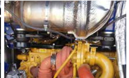
Tier 4 Final / Stage 5 - Caterpillar C4.4 129Kw (173HP)
