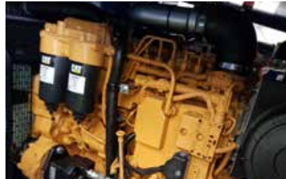
LRC Engine - Caterpillar C4.4 98Kw (130HP)
