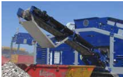
Magnet Head Drum and Chute (Heavies) - Extract ferrous metal from waste stream
