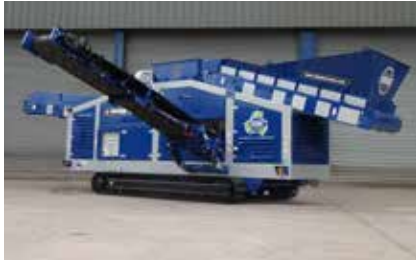
Tracked Mounted - Fully tracked for on-site manoeuvrability
